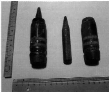
Bullet with a core of depleted uranium found in the nose of specialist of A-10 assault from the US Airforce, analysed in the Institute of Nuclear Sciences "Vinca"
